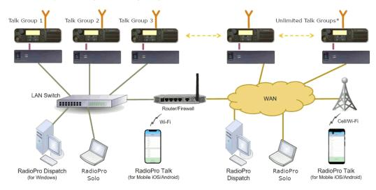
\* Max 80 Clients connected to 1 Gateway. Max 70 Gateways connected to 1 Dispatch Client.
